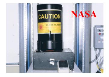
The Micropulse Lidar (MPL) has one measurement channel that records backscatter signals in 300 meter range bins, with the lowest valid range bin beginning at 120 meters above ground level, up to 20+ kilometers. The primary quantity obtained from this signal is the real-time reporting of the lowest detected cloud base in meters, obtained from 60 second averages.
