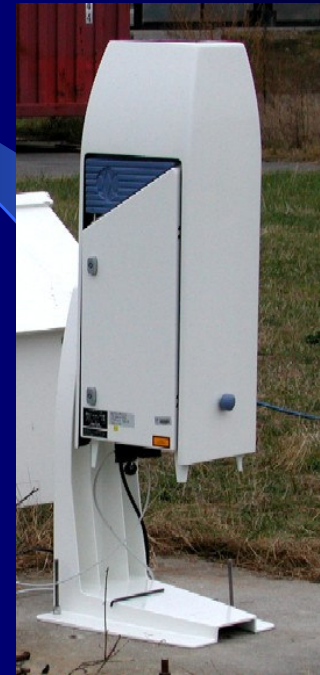
Ceilometer ( \beta lidar @ 0.9 \mu m)
