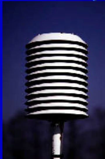
Ventilated shield for temperature and humidity sensors
