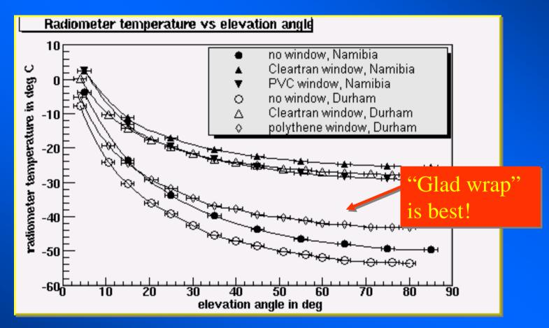
Expected elevation angle dependence is more contrasted using the polythene window, the "Glad Wrap" cling film.
